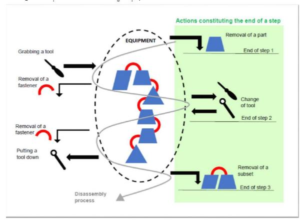
In this example, all the actions carried out (listed on the left and right) can be broken down into three stages. Thus, only the removal of a part, the removal of a sub-assembly or a tool change constitutes the end of a step. On the other hand, the following do not constitute the end of a step: gripping a tool, removing a tool, removing a fastener, and partial disassembly of a pipe or sub-assembly.
